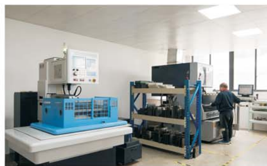
慢走丝 Slow-feeding NC wire-cut machine
